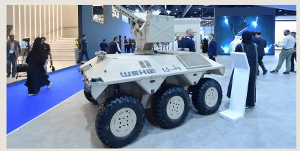
Equipped with a 6x6 all-wheel-drive system, fully independent double wishbone suspension, and differential locks on all axles, WSHG delivers unmatched off-road performance. The platform's switchable two and four-wheel steering enhances stability at high speeds and facilitates tight turns at low speeds, providing operational flexibility across various terrains. MCAV0014 ALHEDA lightweight
