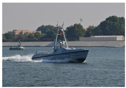
built with fibre mixture and equipped with X band radar, day and night thermal cameras, and a sophisticated command and control system. The UAE MoD's Unmanned Sail Boat (AL SHERAA) added a wind-powered touch to maritime surveillance, equipped with a weather station, navigation radar, and stabilised electro-optic and thermal cameras.
