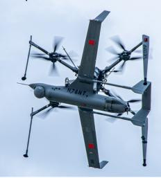
Integrator VTOL is uniquely designed to operate as a portable system in tight quarters, such as ship decks, and in challenging maritime conditions with high seas and gusty winds.
